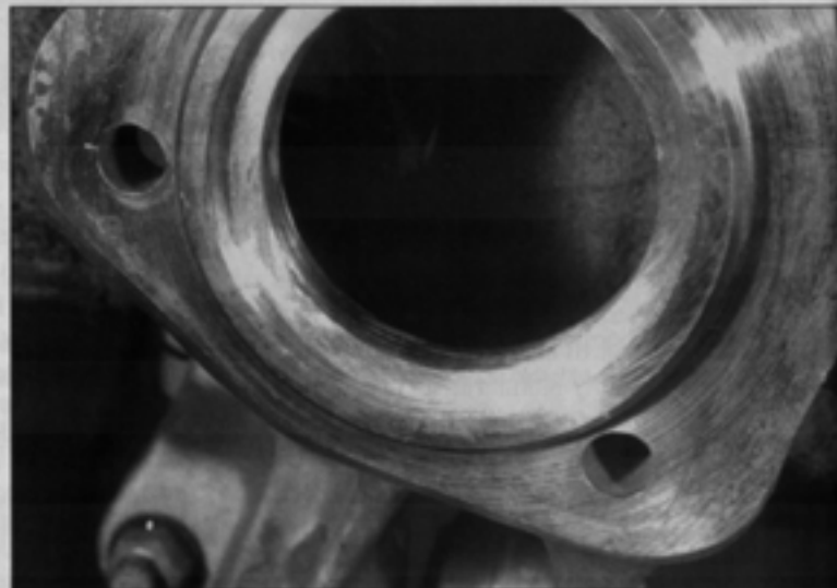
This job turned out quite neat because of the special abrasive wheel Leon used. However, using a carbide burr is just as functional.
