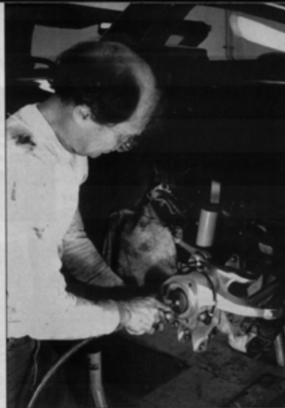
The last nasty task is relieving the outermost part of the knuckle's inside diameter.
