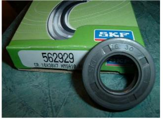
92rohcp decided he did not want to replace his output shaft seal with the old carbon face design used by the original supercharger manufacturer. Here is the new output shaft seal take note of the new part #
