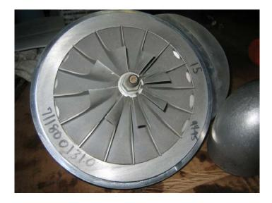
• Remove the 6 bolts and e brackets which secure the compressor housing onto the gear case. Be extremely careful, the compressor wheel is very delicate and can easily be damaged. NEVER lay your supercharger with the compressor wheel down.
