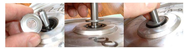
Another noted difference in the SQ is the cover to the impeller has an orange gasket (seal) and a small lip for it to fit into, see below:
