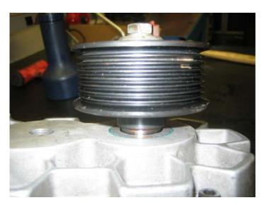
• Re-install the key and pulley. Use impact gun to secure bolt or secure using strap and socket wrench. Be sure pulley is installed with longer nose toward the compressor.
