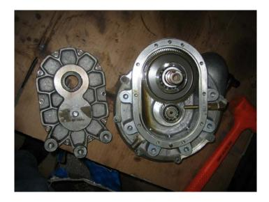
• With care and patience, remove the front cover. There are two dowels which align the front cover to the gear case. Once these clear, the housing will have a tendency to rotate/tilt – do not let it tilt! Pull straight up on the housing, be sure you don't jerk it such that the compressor housing and gear case separate otherwise compressor wheel damage may occur.
