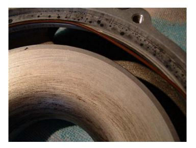
The output shaft seal (compressor seal) was hard to get out. I could not do it with the rubber hammer. I used the press and even that took a lot of force. Remember, this is a different seal than the others (for the V1) seen before.
