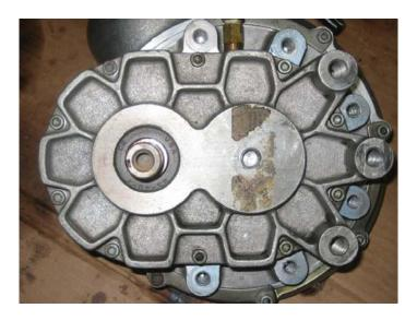
• Remove the 10 bolts which secure the front cover to the gear case.
