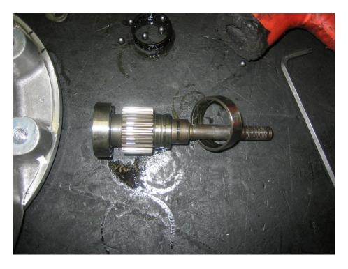
Here's what you're left with if you're not careful, note the ball bearings everywhere! A busted bearing and an inner race that's still on the shaft. No big deal if you're going to replace the bearings.
