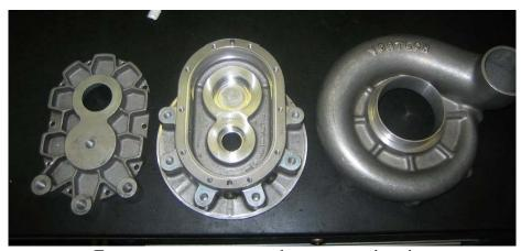
Front cover, gear case, and compressor housing
