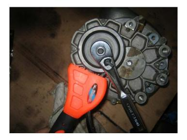
• Remove pulley. A strap wrench may be used if an impact gun cannot be found (but you needed one to remove the compressor nut so you've got one, right?). Using the strap wrench, hold the pulley secure while loosening the pulley bolt.
