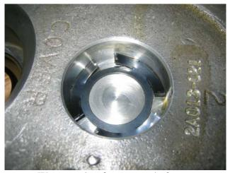
Wave washer for output shaft.
