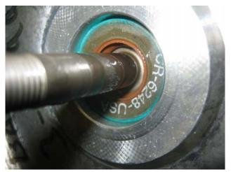
If installed without an expansion cone, the shaft OD is too large to fit through the new seal ID.
