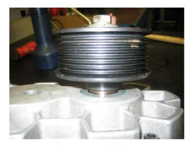
• Note pulley orientation, the long nose points TOWARD the compressor. Bolt is a standard right-hand thread.
