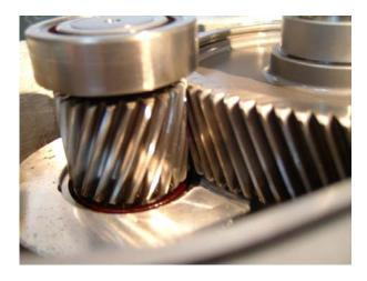
It also appears there is a different style seal for the output shaft, it has a metal in ring that has a hard plastic outer seal that is spring loaded. The plastic part seems to make a seal with the spacer that is between the impeller and the outer gear case. This is not at all like the v-1 units.
