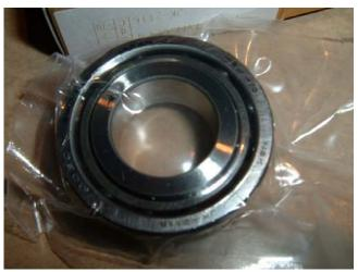
To orient the high speed bearing is very, very easy. The outer race on the thrust side of the bearing will be thicker, that side should face outward or away from the gear. So both bearings thrust sides outward. You will see this on your [supercharger manufacturer] bearings when you disassemble, they will say thrust on that side facing out. So another way to put it is the thicker side thrust side of the bearing will face down into the bearing cups on the gear case and the cover.
