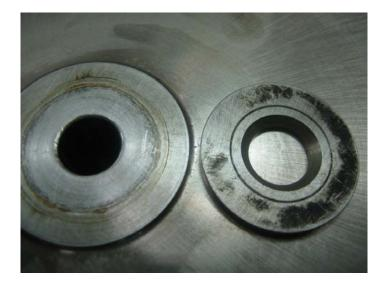
• When both shafts are free from the gear case, place the compressor wheel in a safe place. Note that there should be a washer between the gear case and compressor wheel. This washer has a chamfer on the ID, note the orientation! The washer must be re-installed with the chamfer facing down, away from the compressor wheel.
