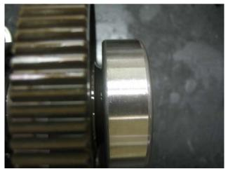
Extremely tight clearance between input gear and bearing.
