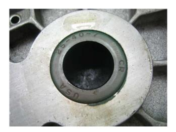
• Input seal is installed so that it is flush with the front cover. Use a flat object to ensure that the seal is installed evenly and to the proper depth.
