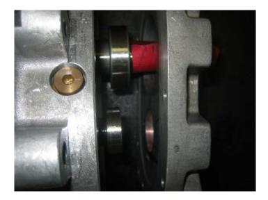
• Place gear case and shafts on side. Using your cone again, place the cone through your input seal, large end toward the input shaft. That red section is the cone I made from a manila folder.
