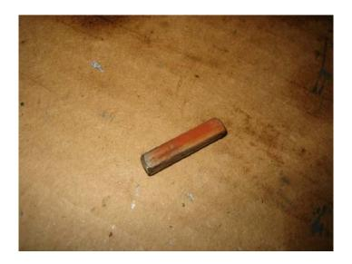
• Be sure to remove key once pulley has been removed.
