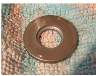
The spacer or washer on the SQ is different, it does not have a chamfer on it. However, it does have a groove in it that faces down toward the gear case.
