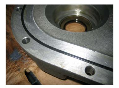
• The large O-ring may come up with the front cover, be careful not to damage this seal as it may be re-used. Check ring for cracks or pinching. After re-installing my supercharger, I see that it is still leaking from the casing. I believe this o-ring is no longer providing an adequate seal for the housings. I plan to replace this o-ring in the near future.
