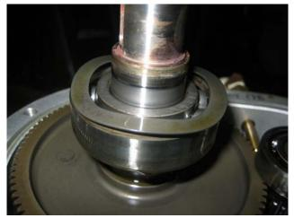
Wave washer for input shaft.
