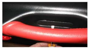
Using a small screwdriver, pry out the cover over the screws behind the door pull The 3 tabs on this piece reinstall at the bottom.
