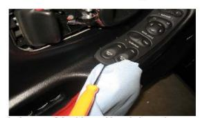
Pry up on the bottom of the drivers side switch panel to remove.
