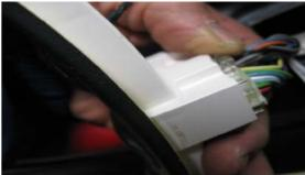
Depress tang on connector and unplug connector for the door switches.
