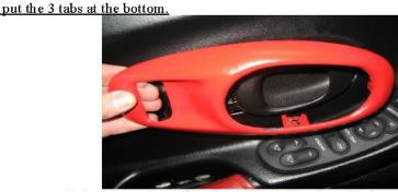
This picture shows the tabs you are releasing with the screw driver. There are 2 to the rear of the bezel that it takes force to release.
