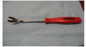
This is a panel removal tool available at any parts store. This is used to remove the doorpanel clips.
