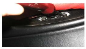
Using a #30 torx screwdriver, remove the 2 screws behind the door pull.Make sure when replacing the piece covering this area you
