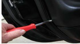
This is the approx. position of the first retainer. Work your way around the bottom of the panel prying the clips loose. There are 7.
