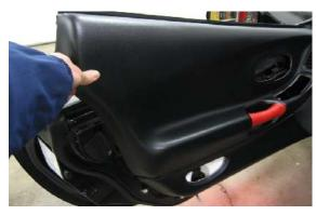
Grab the door handle and lift upwards. It is a press fit so it will take moderate effort. Start at the front of the panel and work rearwards. It may help to firmly smack the upper edge while pulling up.
