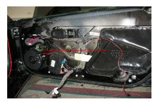
This shows the routing of the wires. Use the factory straps to hold wiring in place. Next step is to route wires through the doorjamb.
