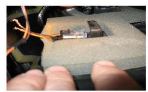
This shows where to tap into the footwell lights. If your still using the footwell lights dont cut the wires, just tap into using the supplied wire connectors. You can also strip the insulation and solder in the wires. Your lights should now work! Make sure the lights arent timed out!!
