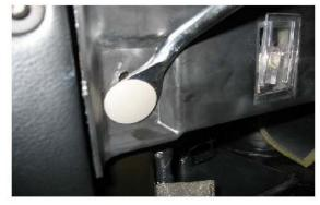
Using a panel removal tool remove the 2 retainers holding the panel above each footwell where the lights are. This is the light you will tap the wires into
