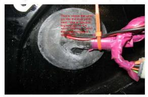
To pass the wires through to the doorjamb you can poke a small hole in the boot, pass the wires through and silicone shut. Or you can unwrap the pink coathangar to aid in routing. This will route the wires into the foottape,pass the wires through then retape.
