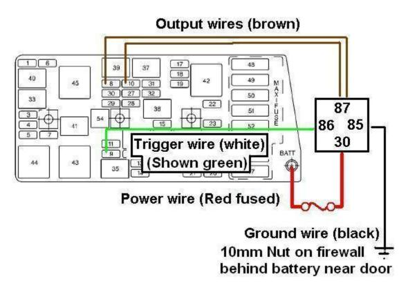
Tap the fuses as shown using the fuse taps supplied with your harness. The leg of the fuse will slide through the tap and back into the fuse socket. The fuse may not seat completely, but as long as you have good contact it will work as
