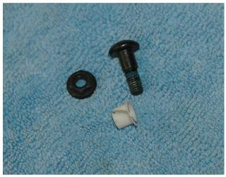
3. With the headlight tilted down, remove the 10mm nut that holds the headlight lifting arm to the headlight motor. Disconnect the headlight bulb sockets and remove the headlight (picture shows the placement of the nut without the headlight.
