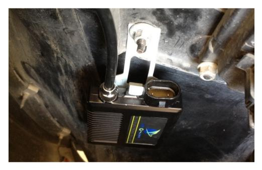
b - use the supplied double-sided tape in the small ziplock bag to adhere the ballast to a clean flat area of your choosing. (make sure the area is clear of the headlight when it moves up and down and the wires will not snag during this motion)
