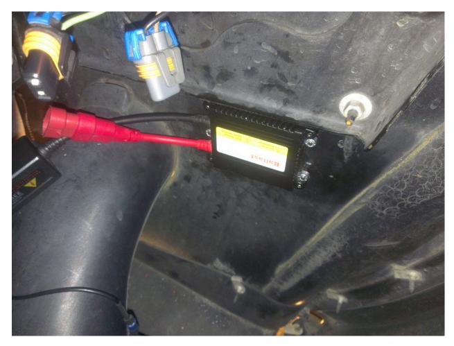
3. Connect the Factory low beam connector directly to the ballast. You will need to plug the ballast the connector in backwards to get correct polarity. When done correctly, the locking clips will be on the opposite side of the locking tab.
