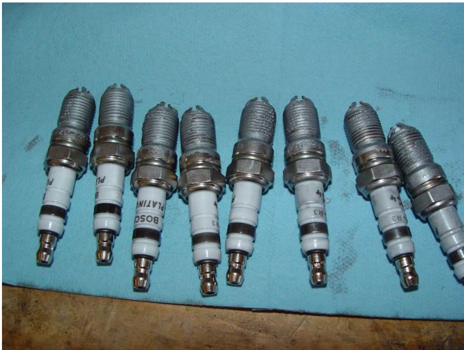
Fig. 10 All the plugs with anti-sieze on them.
