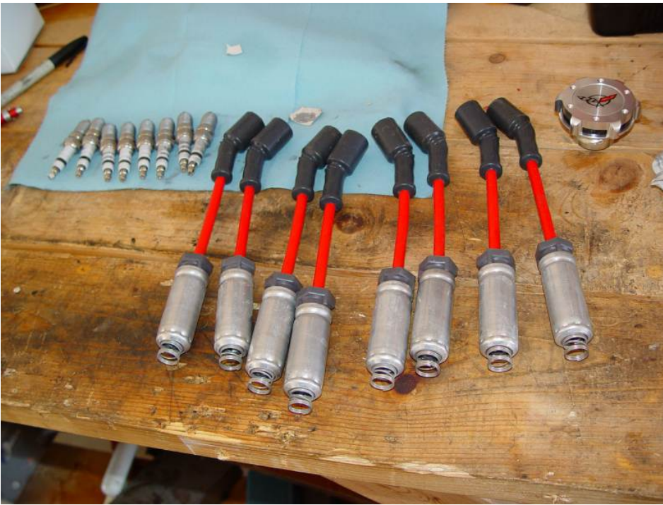
Fig. 12 All plug boots greased, spark plugs with anti-sieze, ready to install.
