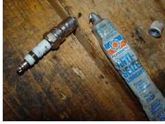
Fig. 9 Put a dab of anti-sieze compound on the plug thread and coat the plug thread and bevel evenly using your fingers.
