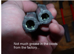
Fig. 11 The factory did not put a lot of grease in the new plug boots...
