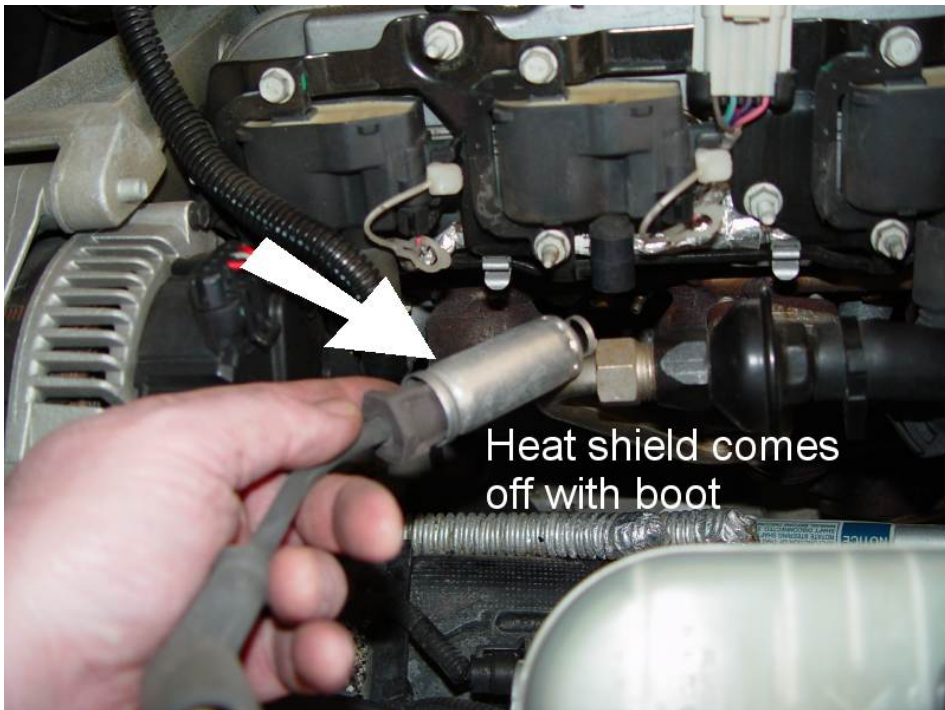
Fig. 6 I pull off the heat shield and the boot all at once.
