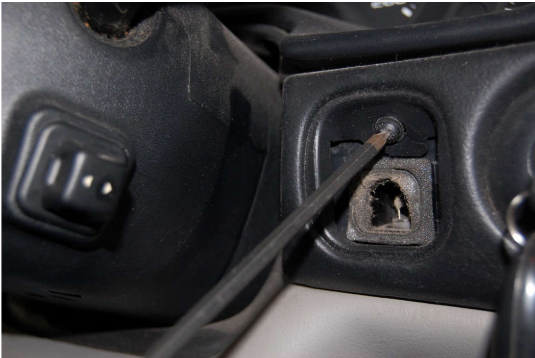
A plastic wedge makes it easy to remove the in-car temperature sensor bezel.
