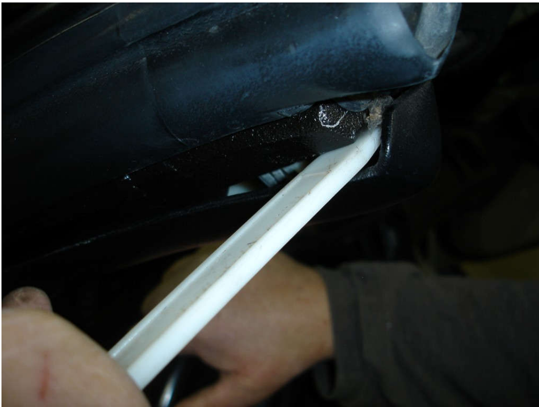
The windshield pillar covers on both sides of the car are removed using the plastic wedge.
