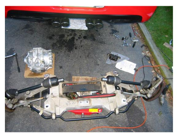
Get out your drain pan, pull the drain plug on the underside of the diff, and drain the fluid. Remove the tranny mount from the rear diff (2 15mm bolts on the underside of the diff). Undo the 2 13mm bolts on the top of the diff, and the 3 15mm nuts on the sides and bottom. Yes, there are 3 - watch for the one that's buried on the underside.
