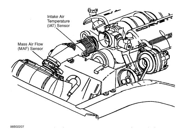
Fig. 4: Front Of Engine Compartment Courtesy of GENERAL MOTORS CORP.
