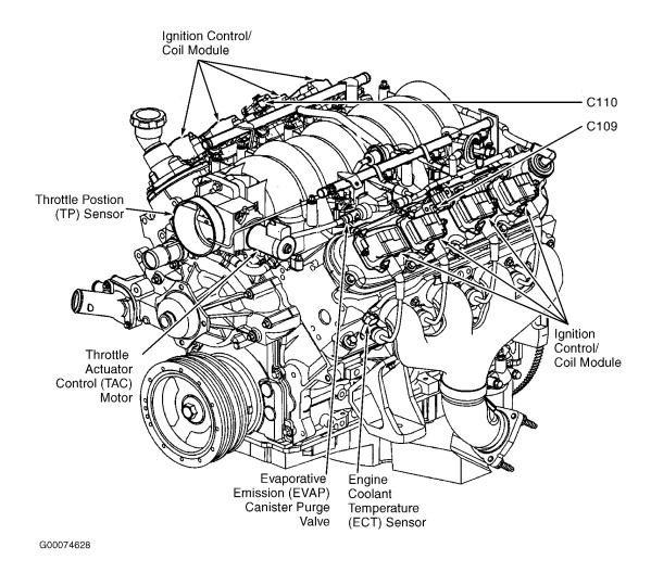
Fig. 3: Left Front Of Engine Courtesy of GENERAL MOTORS CORP.
