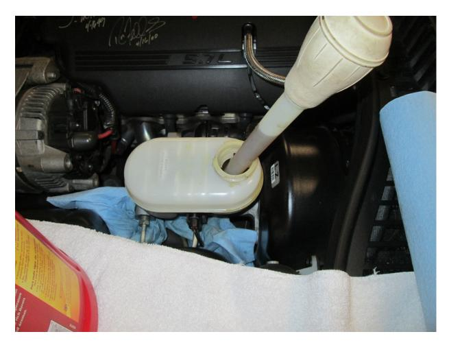
• 12x12 aluminum baking pan placed under the MC to catch fluid when lines disconnected from MC.
