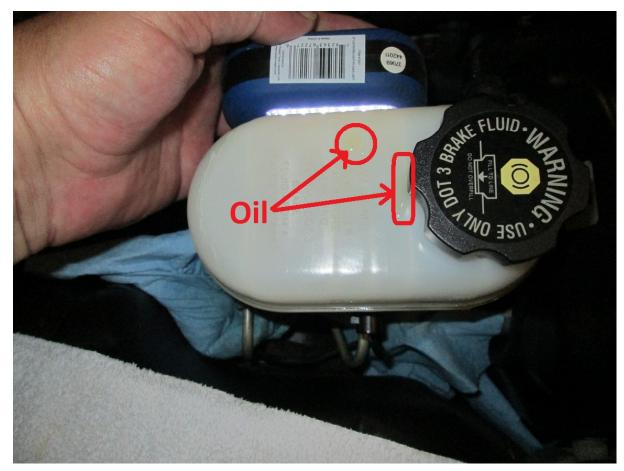
• Close inspection revealed fatigue cracks in reservoir.
