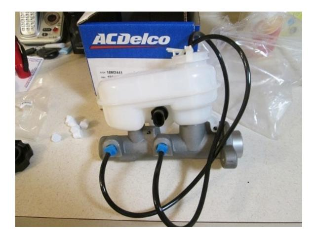
• Clamp MC in vise, service with oil and actuate the MC until there in NO air in the oil "bench bleeding". It took me apprx. 30 cycles to remove air.
