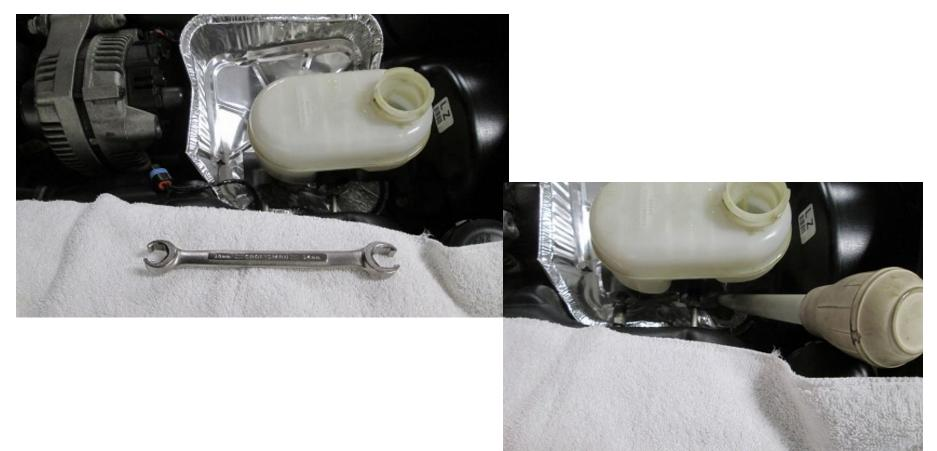
• Brake Master Cylinder removed.
