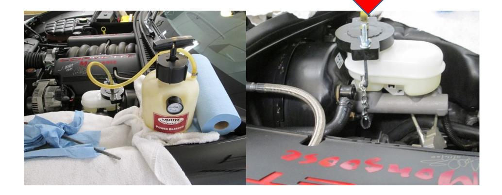
Pressure system bleeding using the Motive Bleeder. Unit serviced with oil and pressurized to 10 PSI.
