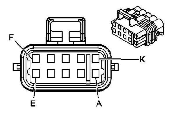
**PCM Connector C1 End View** This connector is Blue for 1999-2004 (For Reference Only. You will be making the connection at the Clutch Pedal Position Switch)
