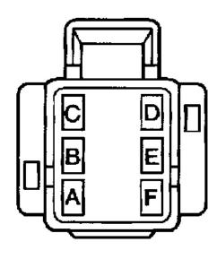
Fig. 1: Identifying Windshield Wiper/Washer Switch Pigtail Harness Connector C219
