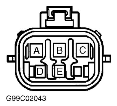
Fig. 2: Identifying Wiper Motor Connector Terminals Courtesy of GENERAL MOTORS CORP.
