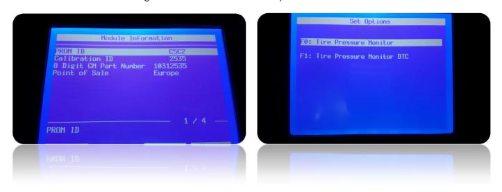
If you prefer DIC to show RFA DTC codes, here selecting F1 you can set the option enabled. Unselect for disabling DTC codes from tire pressure monitoring.
