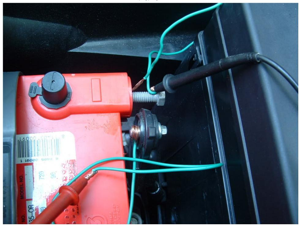
When you initially connect the AMP meter in the circuit, the current draw will be high. Some where around 8 amps. As the BCM determines that the car is secure, it will start dropping off loads and go into the SECURITY MODE and Sleep Mode. As it drops off loads you will see the battery current drop down from 8 amps to around 2-3 amps them in the milliamp range.
