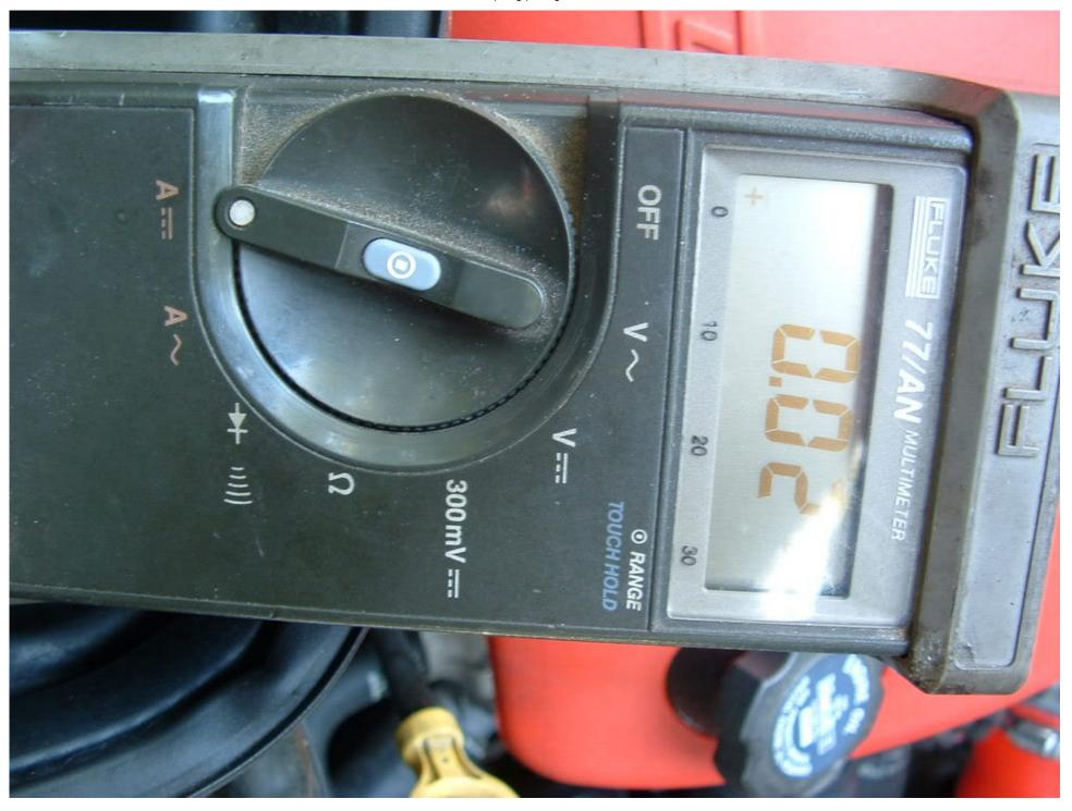
With this small current draw and a properly charged battery in good condition, your C5 should be able to sit idle (**without a battery tender or battery charger**) for at least 3 weeks if not longer. My ZO6 has set idle for 30 days and started normally after that period.
