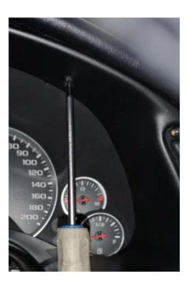
10. Then remove two screws (7mm socket) securing the lower part of the cluster
