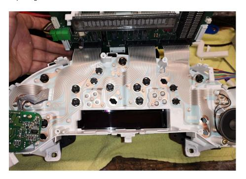
17. When I installed LED's I got the cluster connected like this and checked the LED visibility before I put the cluster back in the car .
