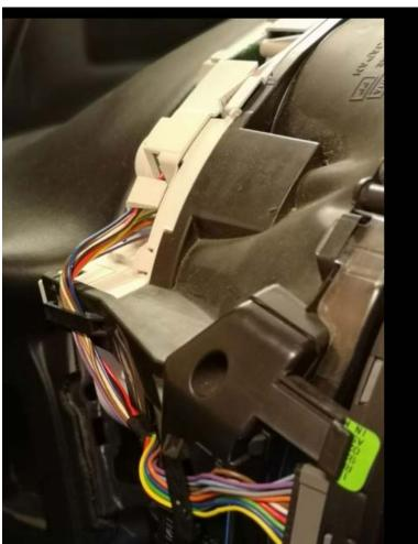
14. When the cluster is out like this it is very easy to disconnect the main cluster connector . When this has been done the cluster is available for several operations ( 15 & 16) <: o)
