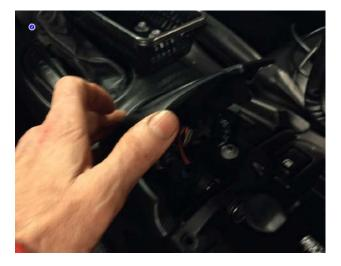
Remove the TC connector and the plug with 12 volt supply to the cigarette lighter in the console
