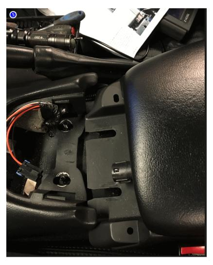
Twist carefully front part of the console like this and disconnect the connector for the gasfuel door open switch .
