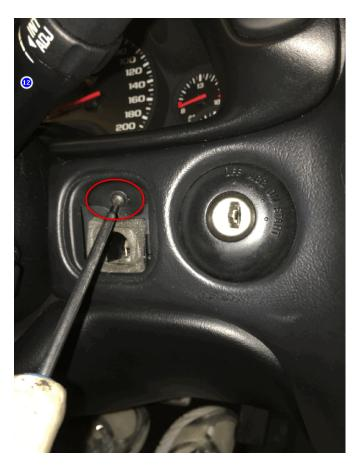
Insert the ignition key and switch ignition key (with BATTERY DISCONNECTED) and pull the gear selector in back position .
