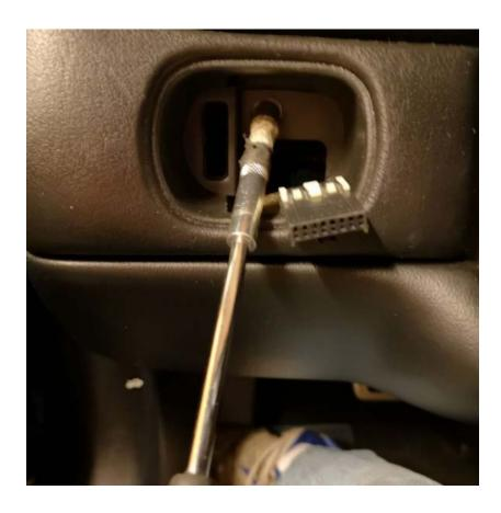
2. Remove 2 stk torx screws at the bottom side of the knee bolster
