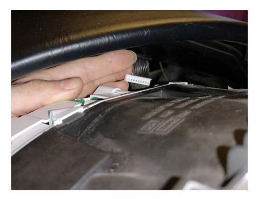
13. Tilt the steering wheel and lift the cluster upwards carefully on the left side off steeringwheel
