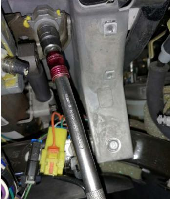
8. When both nuts are removed, the steering column column drops down a bit, shown on the photo
