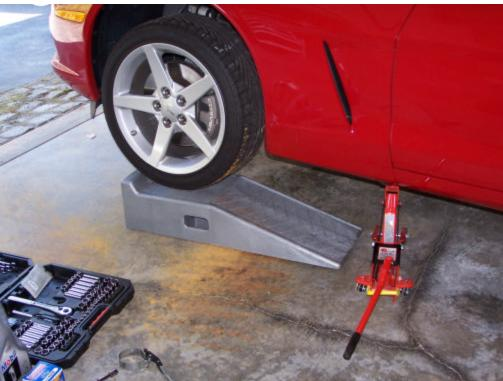
**Step 3.** Get yourself some extra room. Once the jack is in place and the car is up out of the way I will turn the ramp around so that you have easy access behind the tire.
