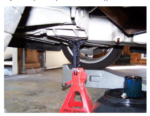
Now that the car is lifted and safely supported you can begin the process of changing out the oil.
