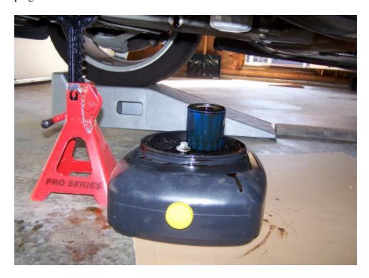
I also prefer to use a drain pan with a screen to catch the oil pan bolt and filter. It's much easier than fishing it out of the oil if you drop it.
