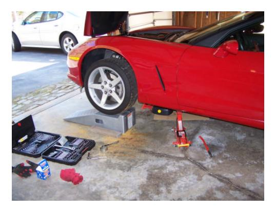
Step 4. Place a jack stand up front under the frame support and lower the car back down.
