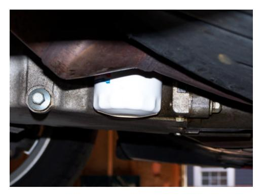
**Step 7.** Using your oil filter wrench, loosen the old oil filter. Once you break it free you can remove it by hand. Plan on oil running down the filter, on to your hands and hopefully in to the drain pan underneath. Once the filter is out, inspect it to make sure that the oil filter gasket came out with the old filter. The last thing you want is an old filter gasket left behind. It will likely cause a poor seal and could cause leaks under pressure.
