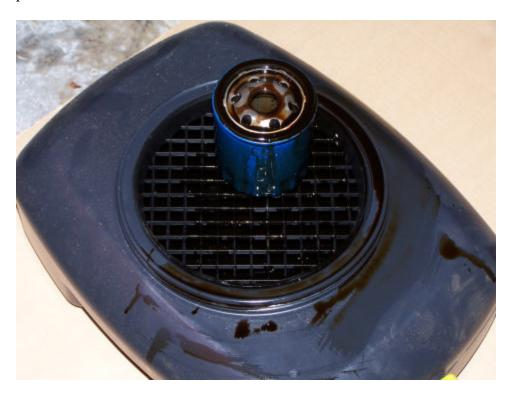
**Step 8.** Wait for all of the old oil to drain out from both the drain plug on the oil pan and the oil filter receptacle. This can take up to 30 minutes depending upon the air temperature, the oil temperature and the viscosity of the oil coming out.
