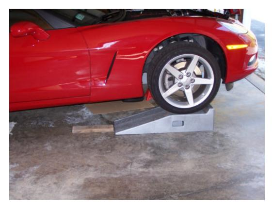
**Step 2.** Get yourself a little more clearance on the driver's side for easier access to the oil drain plug and filter. Once I have the car up on the ramps I take my floor jack and jacking puck and raise the drivers side further. Don't forget to block the rear tires once
