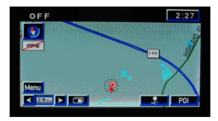
Press the POI button and you will be taken to the Quick POI screen for the navigation system. If the button is highlighted it means that it is showing the icon type on the map. If not, simply select it and it will show the icon on the map and return to the map screen.
