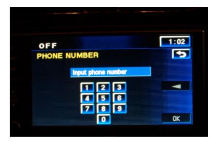
Type in a phone number and hit OK. If you make a mistake, you can back up using the back arrow to the right of the #3 on the keypad. If you don't want to enter a phone number, just press the back arrow (top right) to be taken to the previous menu. Once you enter your phone number and select OK you will be taken to a listing that the phone number points to.
