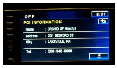
From this screen you can select the pushpin in the lower right to mark the location so that you can return to it later or return to the map screen and mark it as a destination or waypoint using the bullseye (destination) icon or the diamond (waypoint) icon.
