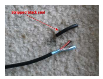
Now that the black seal has been removed, it's time to remove the seals from the actual wires themselves. Put the red wire of the extension cord into the lower end of the wire cutter and **gently** press down to cut away the wire seal. You do not want to cut **through** the actual metal wire. You want to strip away the seal surround the metal without damaging it. Do the same for the black wire.
