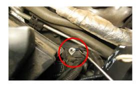
Next connect negative led box lead. Look directly below battery along the frame rail and locate the ground bolt. Use supplied nut and washer to connect. An extra nut is provided in case you drop one. A extendable magnet is helpfull.
