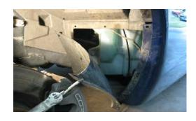
Tie back inner panel to allow access to cove area. If removing cove shields, reach through here with a scraper to detach front of shield. They are held on with adhesive pads.
