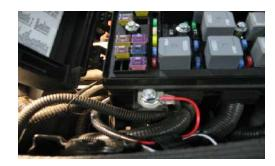
Open underhood fuse box and locate positive terminal. Attach controll box positive lead with supplied nut and washer. Place led box behind fuse box and attach with adhesive pad.
