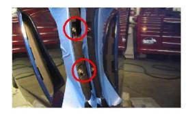
If removing the cove shield for painting, these are the 2 7mm screws that need to be removed. Open the door slightly, tape the paint for protection and remove screws.
