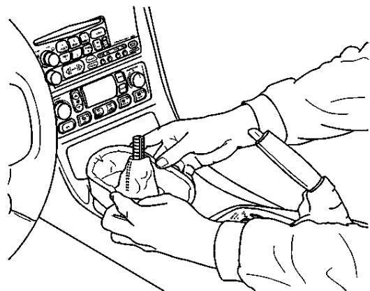
2. Align the shift control boot to the I/P accessory trim plate opening, then press to lock the boot retaining tabs.
