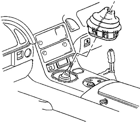
1. Install the shift control boot over the shift control lever.
