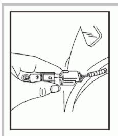
Remove the bulb by pushing in on the tab on the bulb socket and then remove the bulb.
