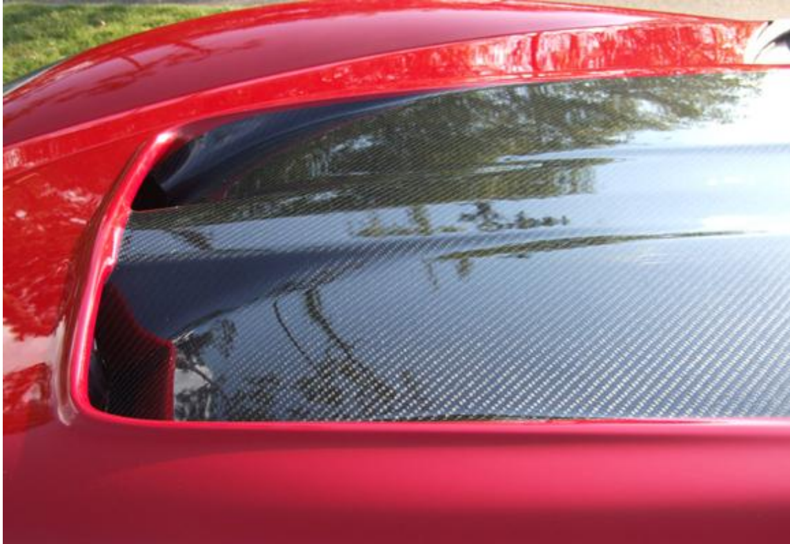
New wind tunnel developed vent extraction lip - the faster the car the more heat extraction - without compromising the driver's view!
