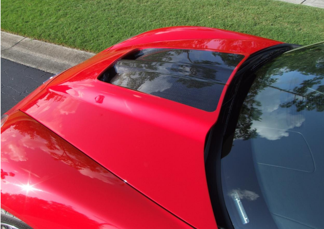
Low profile yet still fits with Magnuson 112, 122 and TVS 2300 series superchargers
