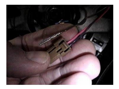
To reassemble -- reverse your steps. Connect the right paddle to its wire connector and mount it with the two #20 Torx (if removed.) Replace the cover with one #20 Torx.
