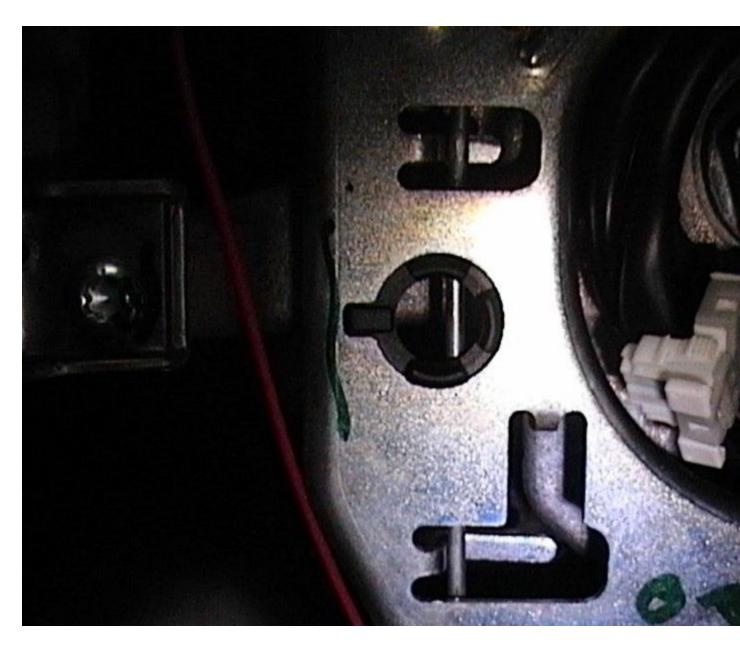
The next photo below shows the spring-wire pushed back that allows the airbag to pull out. You can see the punch inserted.
