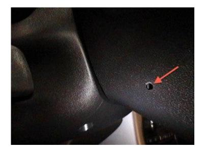
You need to insert a blunt object to press on a spring-wire holding a tapered retaining pin on each side. I used a small punch. A large wire or small screwdriver will also work.
