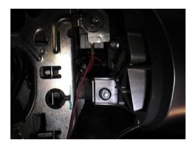
You'll then be able to see the right paddle and its connector. To remove the paddle -- as it may be necessary to unplug the connector -- unscrew the two #20 Torx, unplug the connector and remove.
