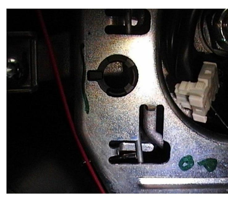
Pull the airbag toward you as you press the spring-wire and it will release as shown below.
