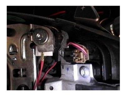
Here's the paddle removed and the brown plug removed (that contains the wires you need to swap.)
