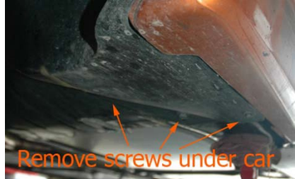
Remove the two 10mm Bolts and one 7mm Screw shown here.
