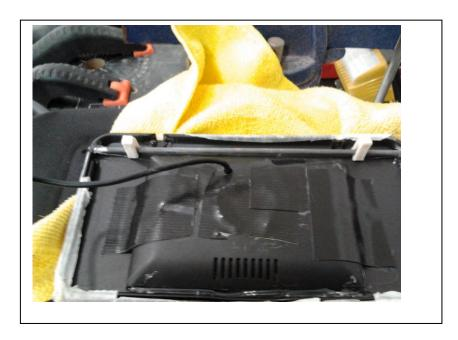
9) The clips are shown in this pic. They are normally used to hold Xmas lights on a house. These are available at Home depot or other hardware stores.
