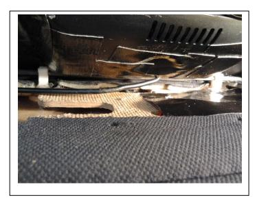
12) Of course, I took it a step further today, and attached rods on each side on the bottom. The clips were also installed. Having clips/rods on top and bottom will keep the cover/monitor very solid on the sunvisor, and easily removable if need be. I did not glue the bottom rods, as the gorilla tape holds it in place very nicely.
