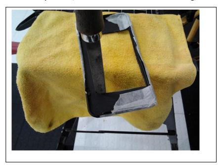
4) The 1/8" holes are drilled on each end on the top, assuring that the rod will be above the monitor. Make sure the hole is as close to the edge as possible. There needs to be a gap between the rod and the back cover so the clips can grab the rod.
