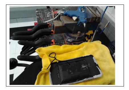
8) The rod is installed, and hot glued in place on each side. The sides of the monitor are covered with Gorilla tape. Note: the clips on the rod will be glued in the sunvisor to hold the cover/monitor in the sunvisor.
