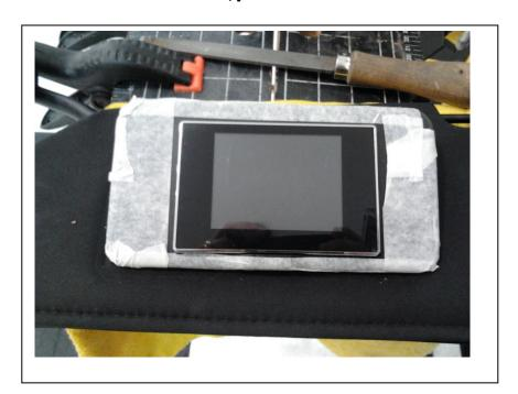
7) With the monitor is in place, hot glue was used to keep the monitor from moving.
