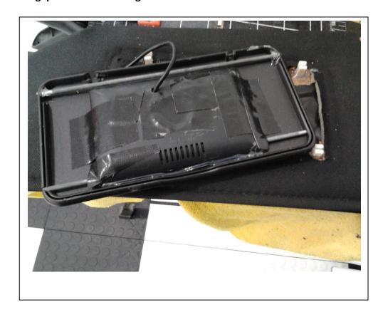
13 The job completed, and a close up picture of the cover mounted on the sunvisor from the side. Notice how tight the cover sits on the sunvisor.
