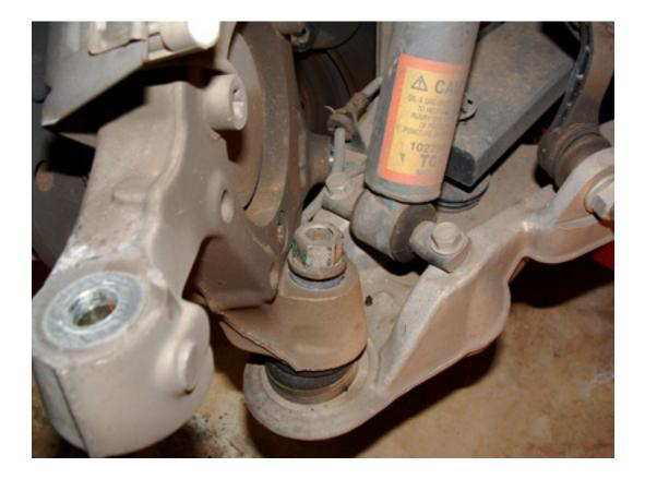
Using a 12" long wooden 2x4, knock the lower ball joint loose by placing one end of the block on the tip of the lower a-arm and hitting it w/ a hammer. (See diagram).
