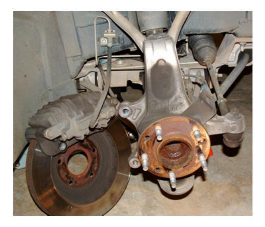
5.) Disconnect the front tie rod (18mm socket) from the knuckle.
