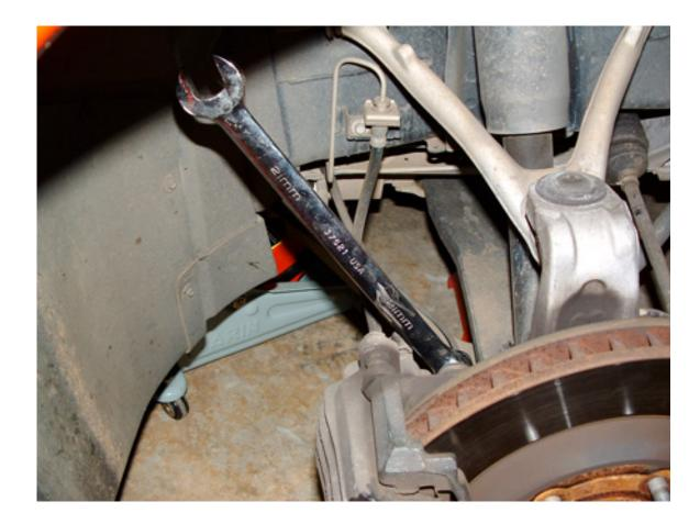
4.) Remove the caliper and brake disc as a whole and use the disc (sitting on the ground) to hold the caliper up to keep tension off of the brake line. (See diagram below)
