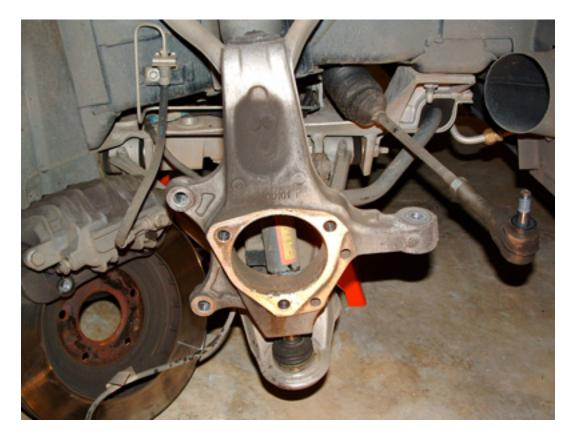
10.) Remove bearing assembly from abs sensor mount. (See diagram below)
