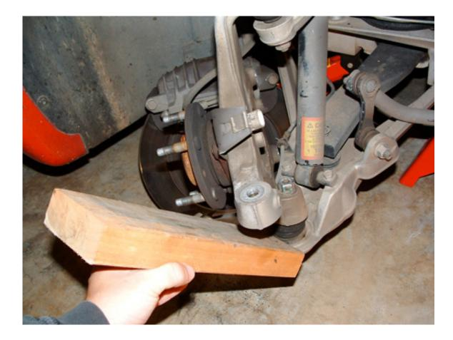
8.) Rotate the upright so that you can get to the three star bolts (T55 Star Socket) which bolt the bearing housing into the upright.
