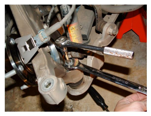
If you don't hold the ball joint shaft with the allen socket, it will simply spin when you install and tighten the nut! <sup>(i)</sup> Once the ball joint has been seated, you can torque the nut w/ a torque wrench.
