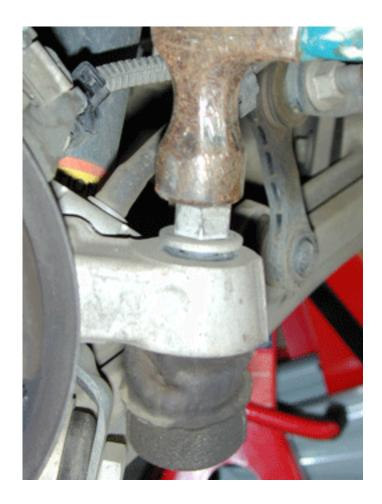
6.) Remove the nut and move the toe link out of the way (See diagram below).
