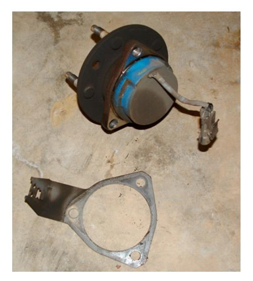
11.) Install the new hub assembly into the abs plate, and install/bolt that assembly back into the knuckle. (Make sure you put the plate back on, like you took it off, with the abs flange pointing in towards the engine. Or, just look at the pics below!)
