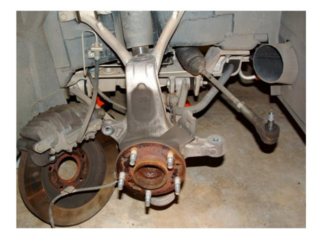
7.) Remove the lower ball-joint nut (21mm) (bottom inside of upright). You may want to WD-40 the threads before you start loosening the nut to ease removal.
