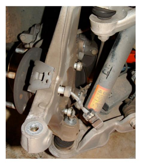
9.) Remove bearing assembly from upright. (See diagram below)
