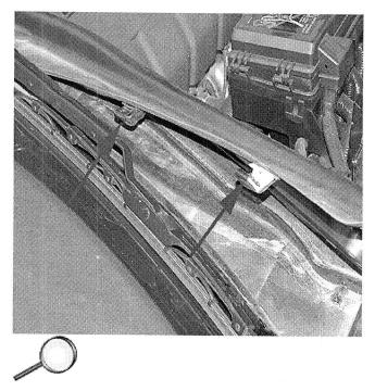
5. Disengage the two hooks that retain the cowl trim panel to the windshield glass on the right side. Lift the right side of the panel as shown to expose the two right clips.
