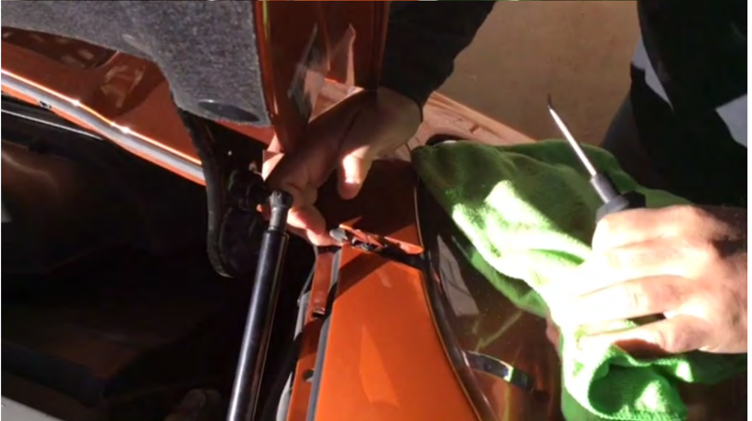
Step #4 Remove the screws holding the plastic wheel well to the front bumper, i think its like 5-6 torx screws.
