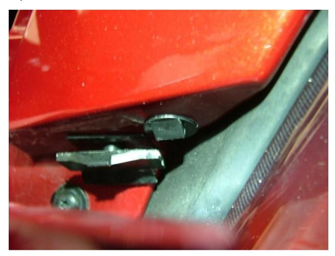
Note: Removing the old clip/locator and inserting new ones can be done without lifting the front bumper cover off the retaining studs, but you will have more room to maneuver if you do slide the bumper cover off the retaining studs.
