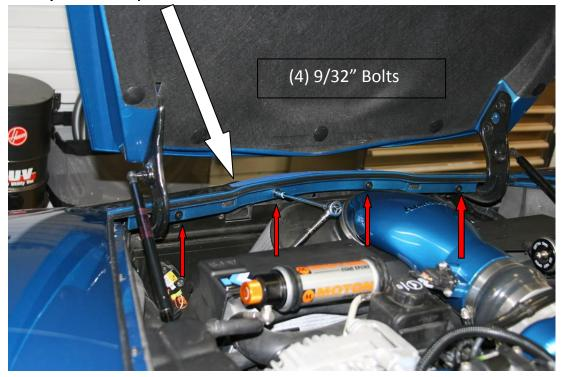
3) Once the 4 bolts are removed, pry the bumper cover off the retained studs.
