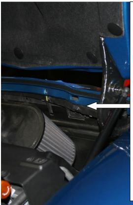
Note: The bumper cover is lifted above the retainer to give better access to the clip. The bumper cover can be lifted even higher, off the frame under the cover so it touches under the open hood, hence why the tape is attached initially on top of the bumper directly under the open hood to prevent paint scratches.
