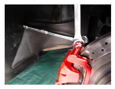
Replacing the rear pads are exactly the same technique, except the shape of the caliper is different.
