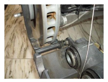
Now, re-install the new clips that came with the new brake pads.
