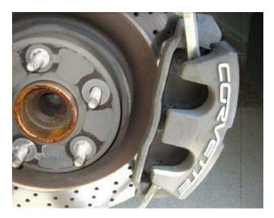
Now, find the bolt at the top and back of the caliper. You will need a back up wrench to hold it steady, while you remove the front bolt as per the pics below. The back- up bolt is 18mm and the front bolt is 15mm
