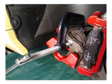
Put some silicone grease on the backside of the new pads, then slide them into place on the clips.
