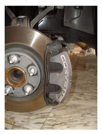
4) To make it easy to remove the caliper from the rotor, use 2 flat head screwdrivers and pry as per the picture. This will compress the pistons into the housing, and make the caliper easy to swing off the rotor. To prevent chipping the caliper paint, wrap electrical tape on the screwdriver shafts.
