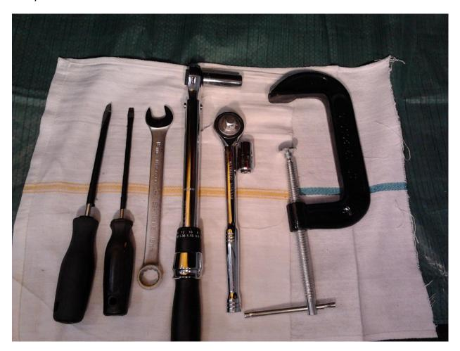
3) Tools Needed: 2 flat head screwdrivers, 18mm Open End wrench, 15mm socket and "C" Clamp, Torque wrench
