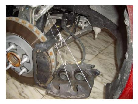
Now, remove the pads by pulling out perpendicular to the rotor. They are not identical, take note of which came from the front and back. The back pads have the thickness indicator attached to it.
