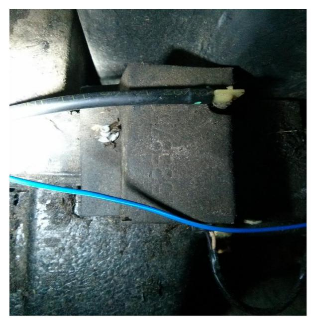
when you flip the cover from right to left you will see the **solenoid**. I used a small flat head screwdriver and a little elbow grease to get the rubber attachments off the black attachments. Very easy, just be careful with the screwdriver and don't tear the rubber
