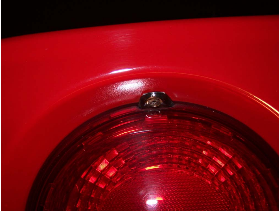
The light is held in place by one T15 Torx screw.
