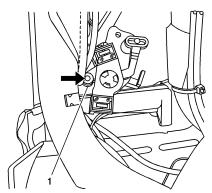
27. Install the folding top position switch and screw (1) if equipped and the interior trim to the top of the "B pillar.
