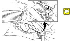
22. Attach the second D-ring and the end of the string (1) to the convertible top linkage.
