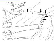
Some customers may comment that the headliner has some wear damage on the outer edges along the upper trim. Condition #2
