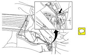
12. Remove the screw (1) holding the D-ring and the string end from the lower corners.
