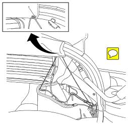
11. Remove the screw (1) from the D-ring on the number 5 bow.
