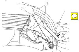
8. Disconnect the folding top rear counterbalance arm spring clips and set the arm (1) aside.
