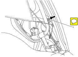
26. Put the string end from the anti-glare cover through the metal ring and attach the end (1).
