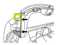
3. Remove the front weatherstrips and retainers from the right and left sides.
