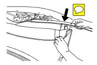
4. Remove the five folding top cover retaining screws from the #1 header bow and remove the retainer.
