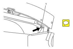
5. Remove the screws in each front corner of the headliner (1) and pull back the front edge of the top cover from the #1 bow.
