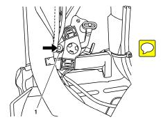
6. If the vehicle has a power folding top, do the following: To gain access to the folding top switch, remove the interior trim at the top of the B pillar. Remove the screw (1) from the switch and set aside.
