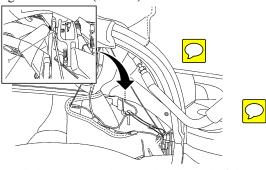
20. Install the screw (1) that attaches the end of the string from the headliner to the convertible top linkage. Note that this is the string with only a retainer at the end.
