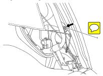
7. Remove the screw (1) from the left and right sides of the string holding the anti-glare screen. Fold the anti-glare screen over the top of the number 5 bow.
