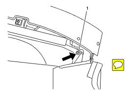
29. Install the screw (1) in each corner of the headliner.
