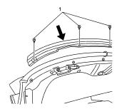
2. Remove the five folding top compression seal panel screws (1).
