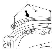
30. Fold the top cover over the #1 bow and install the top cover compression seal panel retainer and screws (1).
