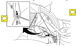
**Important:** Note orientation of the P-clip and D-ring. They must be in this position.
