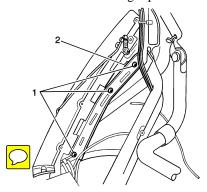
9. Remove the three headliner retaining screws (1) and remove the retainer (2) from the right and left sides.
