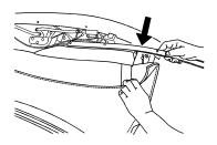
28. Install the headliner retainer and five screws to the #1 bow.
