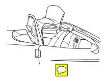
1. Position the top with the #1 bow and the #5 bow up and secure top with the strap.
