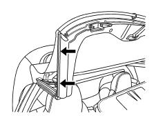
31. Install the front retainer and weatherstrip on both sides.
