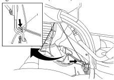
23. Grab the third D-ring and slide the metal ring over the string (refer to the LOWER arrow in the illustration above).
