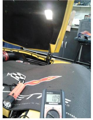
Wait until the light goes out, and you should see the reading gradually reduce to 0.01-0.02 Amps.
