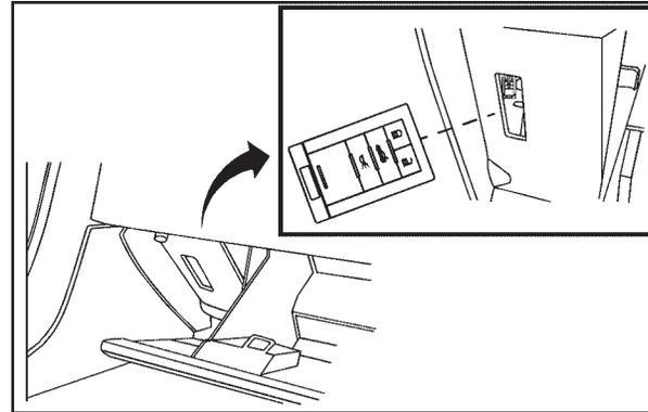
2. Place the new transmitter in the glove box transmitter pocket with the buttons facing the passenger side.
