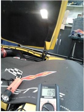
Wait until the light goes out, and you should see the reading gradually reduce to 0.01-0.02 Amps.
