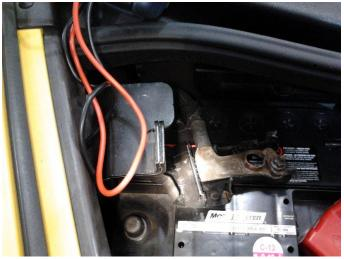
Hook up your multimeter (set for 10 Amps) and connect the red lead on the removed negative battery cable, and the black lead on the negative battery post.
