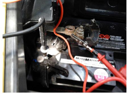
When you initially hook up the multimeter, the under hood lamp will turn on. With the lamp on, the reading will be approx 1.1 Amps, per the attached pic.
