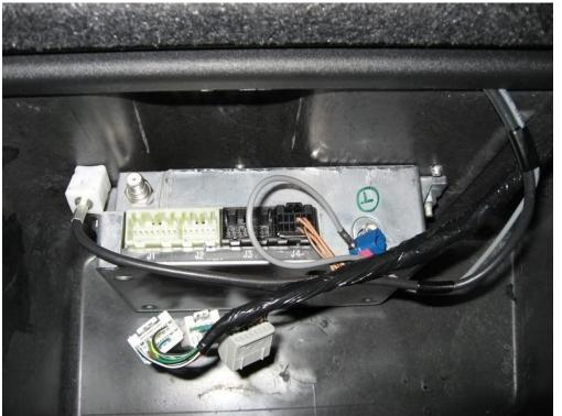
3) Do you leave I-pod or such plugged in to your accessory plugs? Even if the IPOD devise has been unplugged, this device must be removed from the vehicle completely. The devise triggers the Bus to maintain power even when the devise is not powered.
