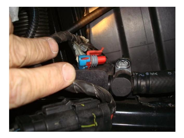
Slide the Vent Solenoid Assy of its bracket. Although it looks like it would slide towards the front of the car it does not. Simply lift the back of the assy high enough for the dog ear to clear the back of the bracket and slide toward the rear of the car. The pic below shows you how it mounts and the dog ear location.
