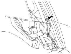
26. Put the string end from the anti-glare cover through the metal ring and attach the end (1).
