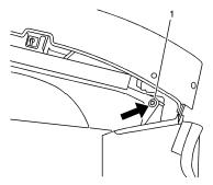
5. Remove the screws in each front corner of the headliner (1) and pull back the front edge of the top cover from the #1 bow.
