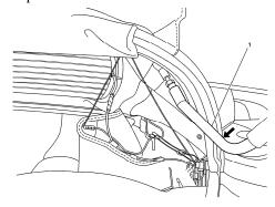
8. Disconnect the folding top rear counterbalance arm spring clips and set the arm (1) aside.
