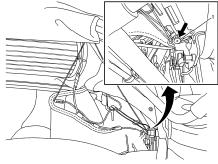
22. Attach the second D-ring and the end of the string (1) to the convertible top linkage.
