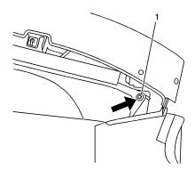
29. Install the screw (1) in each corner of the headliner.
