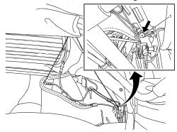
12. Remove the screw (1) holding the D-ring and the string end from the lower corners.
