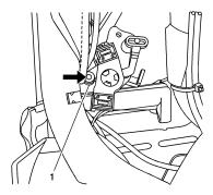
6. If the vehicle has a power folding top, do the following: To gain access to the folding top switch, remove the interior trim at the top of the B pillar. Remove the screw (1) from the switch and set aside.
