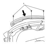
2. Remove the five folding top compression seal panel screws (1).
