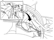
20. Install the screw (1) that attaches the end of the string from the headliner to the convertible top linkage. Note that this is the string with only a retainer at the end.
