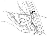
7. Remove the screw (1) from the left and right sides of the string holding the anti-glare screen. Fold the anti-glare screen over the top of the number 5 bow.
