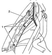
9. Remove the three headliner retaining screws (1) and remove the retainer (2) from the right and left sides.
