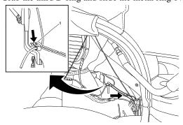
**Important:** Note orientation of the P-clip and D-ring. They must be in this position.
