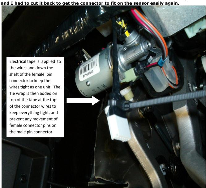
Here's the connector re-plugged into the steering angle sensor....
