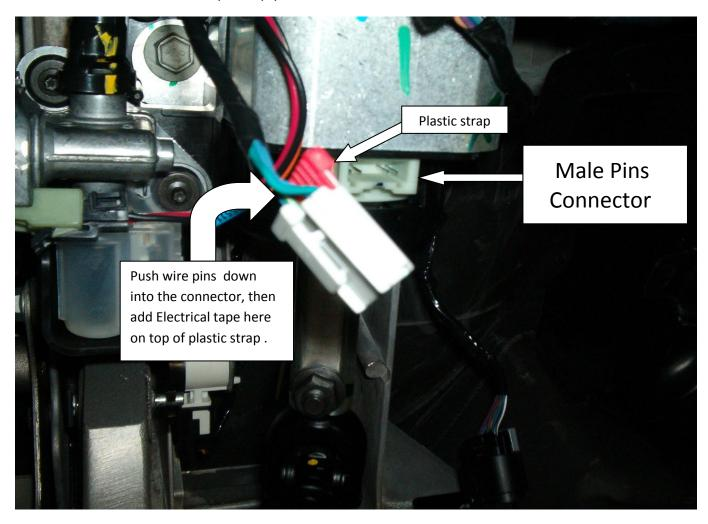
Here's my interpretation of the TSB fix (didn't have a pic). I also suggest putting the zip tie connector to the side not the face as it interfered with the aluminum housing
