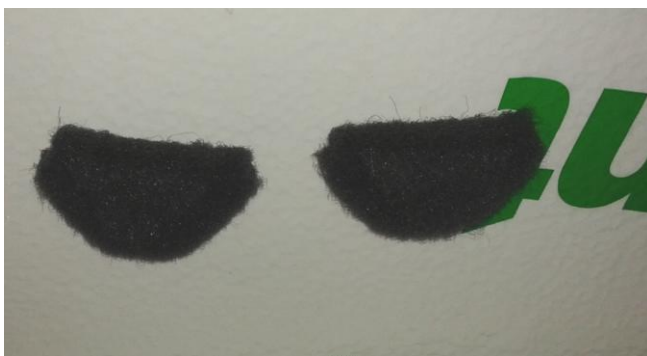
Wood Spacers with carpet (1/4" -3/8" thick) depending on your requirements. (more info on these spacers (#19))
