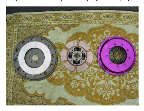
Install the flywheel. 6 bolts, I recommend at least blue loctite. Tighten in a criss-cross pattern in 2 or 3 steps. I did 30, 50, then 74 ft/lbs. At this point, clean the crap out of the face of the flywheel with a clean rag and brake cleaner. It MUST be absolutely clean! While you're at it, clean the face of the new pressure plate and both sides of the clutch disc.
