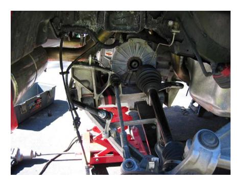
I see a lot of people warning about hitting the firewall with the back of the engine. I don't think this is much of a concern. I watched the back of the intake, and the plate over the driver's fuel rail and they never came close to hitting. I stopped once the top of the rear diff was almost even with the bottom of the tub that hangs down in the back of the car.
