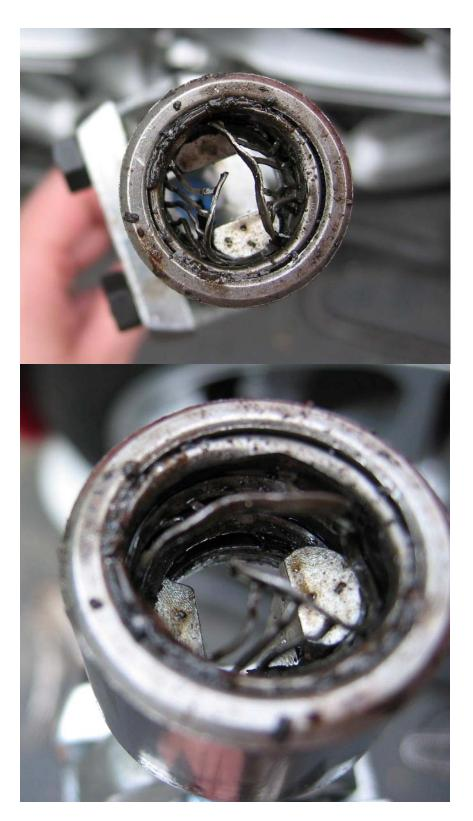
As you can see, the jaws ripped out the center of the bearing (all the little rollers came out) until it came to the outer (facing the rear of the car) lip, where it finally caught.
