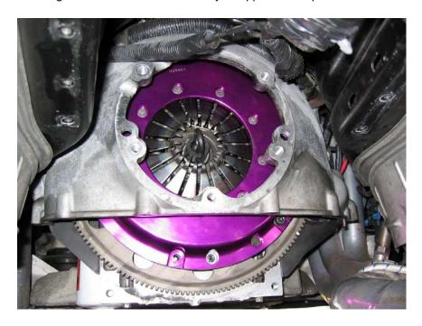
Remove the 6 13mm pressure plate bolts (assuming you have a stock clutch). Be careful, the pressure plate AND the clutch disc will come out when you remove all the bolts. They are fairly heavy too. Remove the 6 15mm flywheel bolts and remove the flywheel. Sorry, didn't take a pic of this part, but basically all you will see is the back of the engine and the crank.
