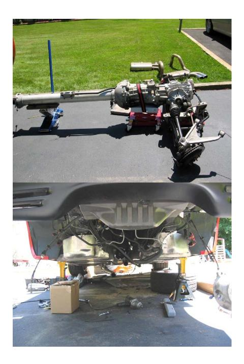
If you have headers that partially block the bellhousing, it's time to pull them. It's not necessary to completely remove them, just remove the 5 10mm bolts from each header flange and swing them out of the way (I used bungee cords to hold them out of the way). Pull the small bottom piece (inspection cover) of the bellhousing (a few 10mm and 13mm bolts).
