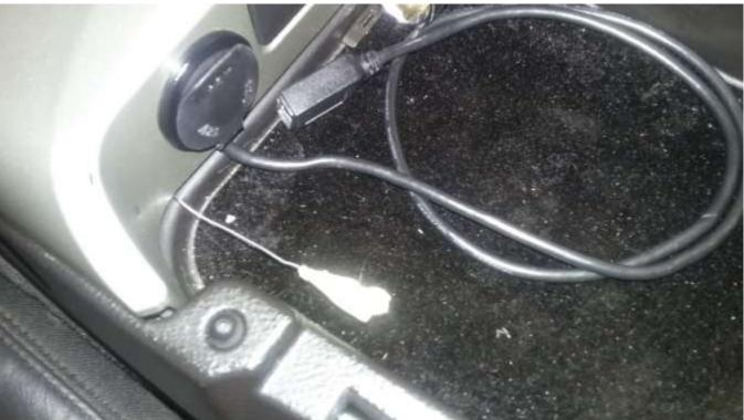
18) Re-installing components is basically reversing the steps. The most important step will be to assure that the shifter pointer is reinserted in the shifter shaft holder. The holder moves up and can be turned in order to get the pointing tab rod back in the cylinder. Once that is accomplished, then the top plastic/rubber boot assembly can be pushed and locked into their holders.
