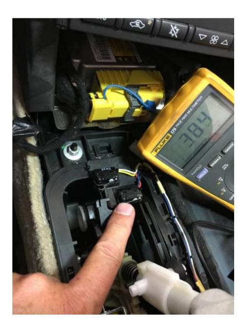
The Normally Open micro switch is 12V 5 amps at 125-250VAC and has a body size of 3/4x1/4x3/8"
