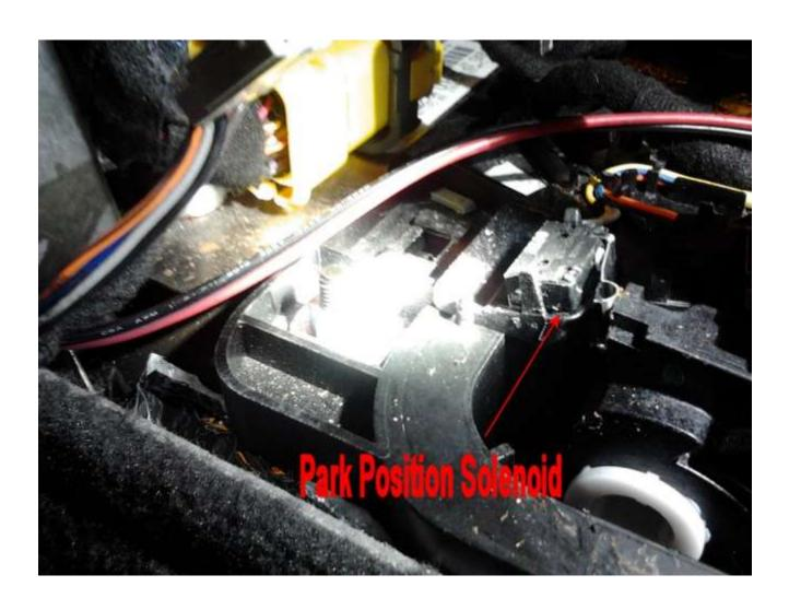
12) Assuming that your transmission was able to be forced out of Park and stuck somewhere around Drive or Neutral. In order to release the Locking Pawl (tab), a small flat screwdriver can be inserted between the locking pawl and the catch, and pried up to get it released. Once this tab is released, then the shifter finger button can be pushed in, and easily moved into the Park position.
