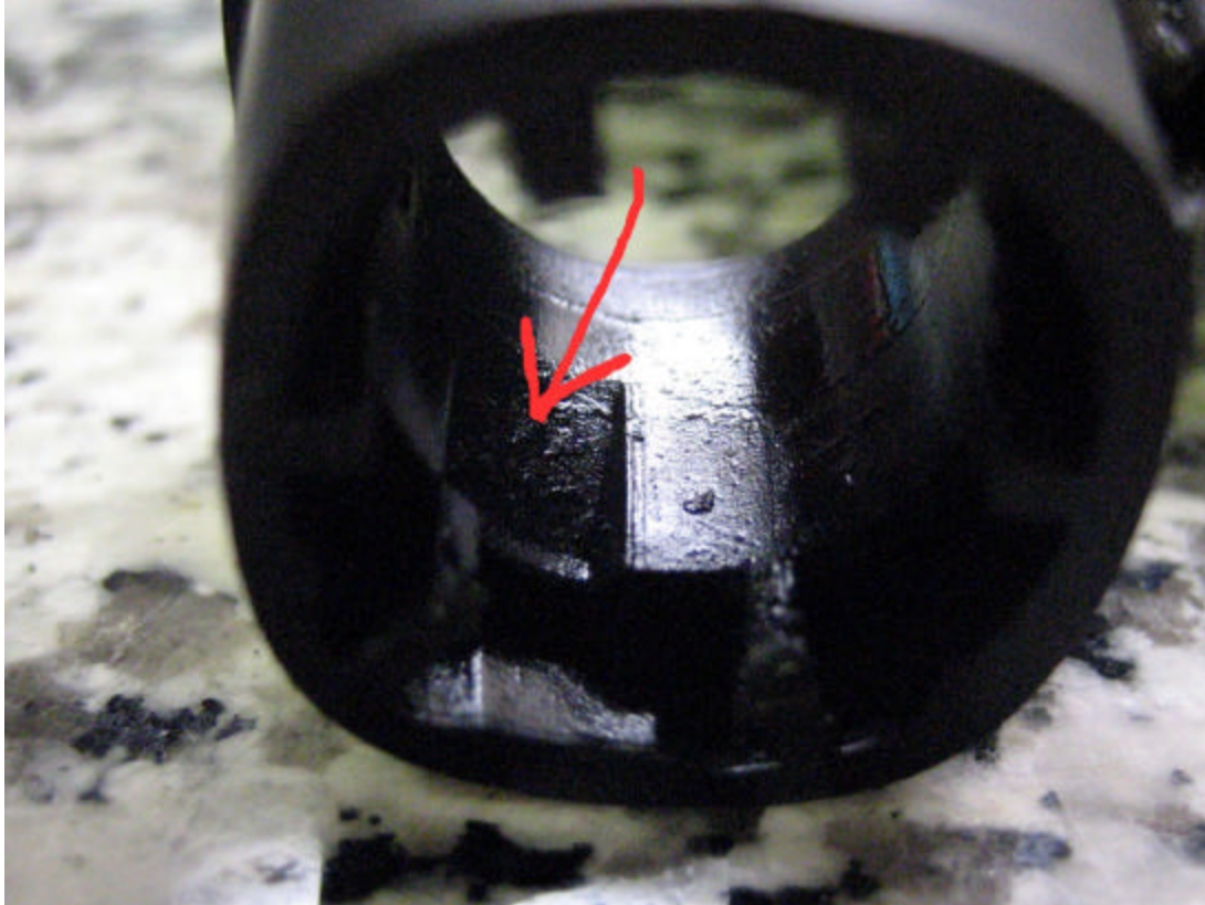
This picture shows deep indentations at the base of the retaining ring where the ends of the shifter prongs lock when rotated to the 12:00 position.
