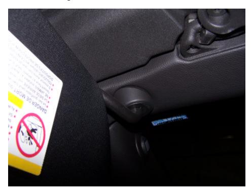
Once the bezel and the assembly are unlocked from the car you will need to pull down on the sun visor arm to remove it from the hole. You may need to work it back a forth slightly to free it from the car. Don't pull down too hard. Firm is fine but be prepared for it to come loose. Now that it is loose from the car you still have the connector assembly to contend with. You may need to reach up inside the opening to free the connector. The connector looks like this:
