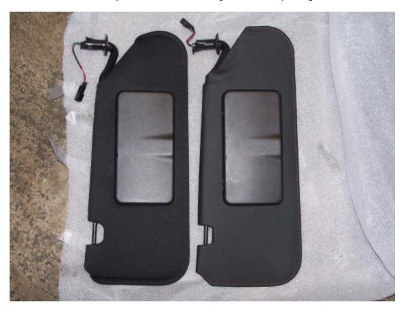
The DSV unit starts with an OEM core and removes the fabric treatment and replaces it with the same high quality leather used in each of the other interior parts
