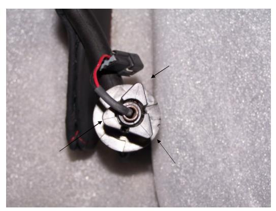
Each corner has a different radius and will match up with a radius on the bezel as pictured here:
