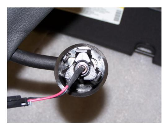
With one tab of the bezel now aligned with each tab of the visor assembly. You should also notice that the base of the bezel as viewed from the side is now flush with base of the visor connector mount. You are now ready to put your new visor back in the car.
