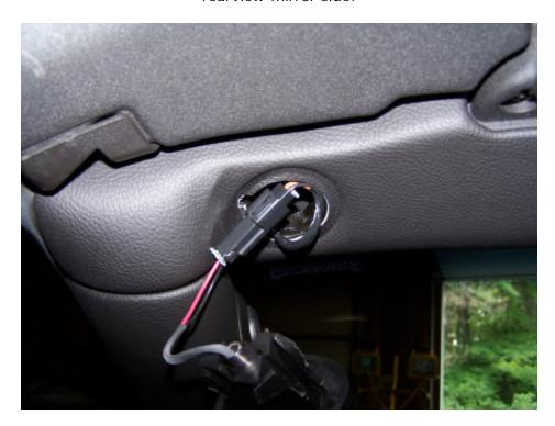
It's time to push the visor assembly and bezel back up in to the frame. There is only one way for it to go back up into the car. You may need to work it a little bit to find the location but try to remember the angle at which the visor was at when you removed it. Once you find the slot for the latch to go into, slide it up and press it firmly in place. You will need to hold it in place and reach for your screw driver. It should look about like this:
