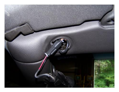
To disconnect the connector you will need your screwdriver again to free the clip from the detent on the mating connector. You can see the slot for the detent pictured below. Insert the screwdriver in the top righthand corner and gently pry forward until the clip is above the height of the small tab. This will allow you to pull on the connector and free the visor.
