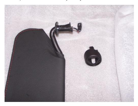
Pick up the new Down South Vettes visor and take note of the shape of the locking mechanism at the connector end. You will notice three distinct shapes to the corners of the connector triangle.
