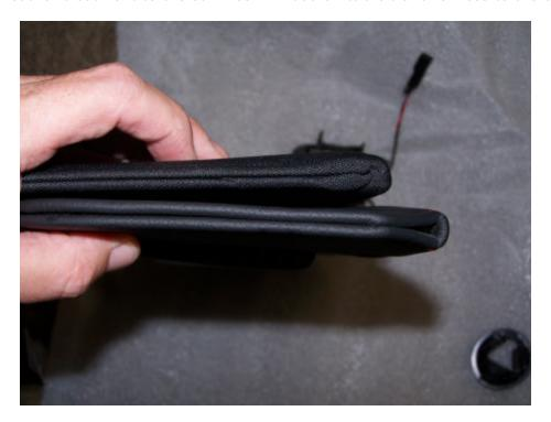
Start the installation by tipping the sun visor down towards the windshield as if you were trying to block out the sun while driving.
