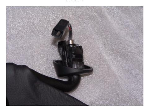
Now you need to remove the bezel from the visor assembly. If you look down at the connector end and bezel you will notice three locking tabs on the bezel that hold it on the visor assembly.
