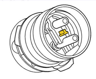
TIP: Fuel Sensor Lock Ring Tool J-39765A is required.
