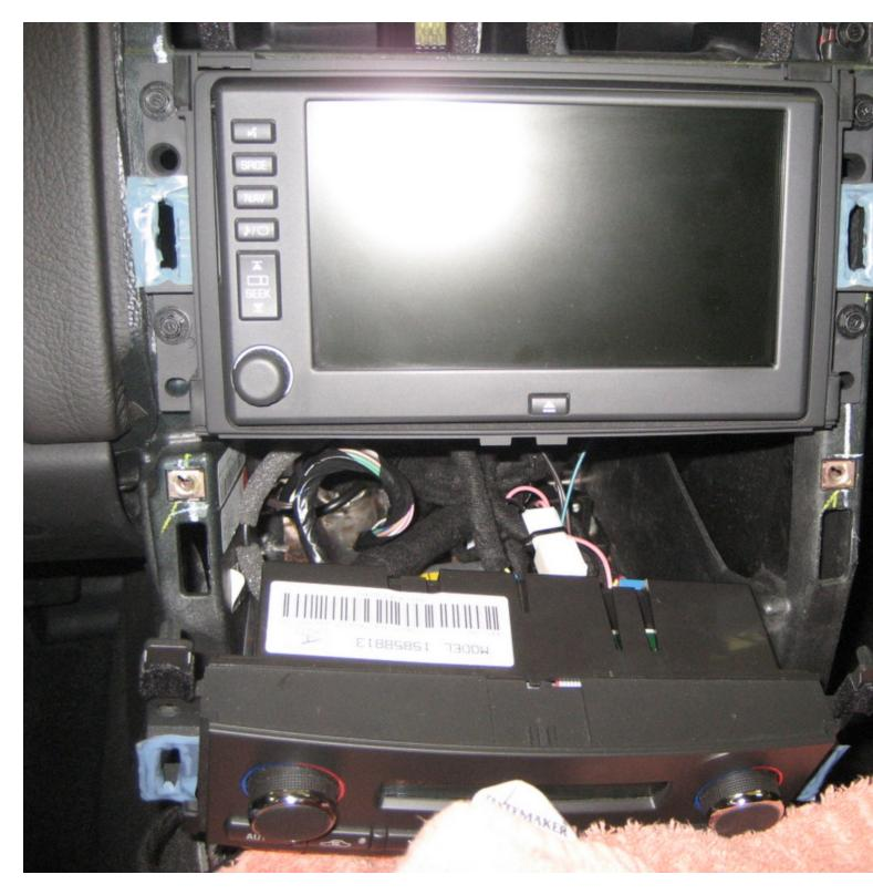
9. Remove the four screws holding the nav unit in place, and pull it out enough to get to the rear plugs.
