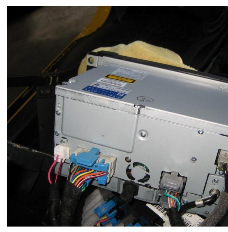
10. The Connector C1 is the 24 pin connector on the left. Connector C2 is the 12 pin connector on the right.
