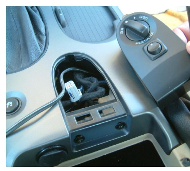
3. Remove the shifter knob. Push down on the leather shifter cover to expose the T-25 Torx screw holding the shift knob in place. Then remove the knob.
