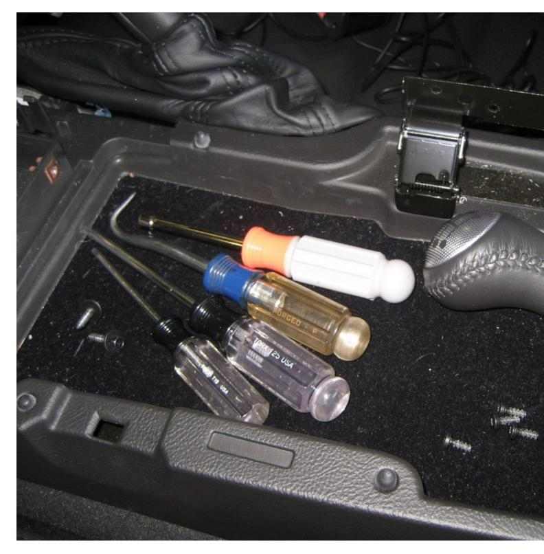
A T15 and T25 Torx driver, a 7mm nut driver, and the I find the bent tool (cotter pin remover) helpful to later remove the power connectors.
