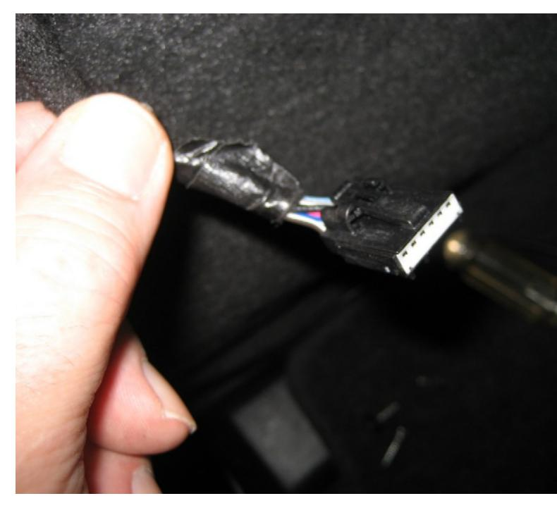
The release tab is on the top in this photo, but on the bottom when inserted into the switch:
