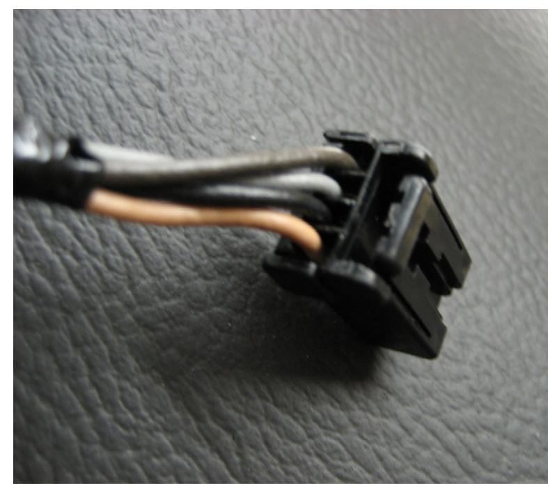
The release tab is on the right in the photo, towards the ground when in the console.
