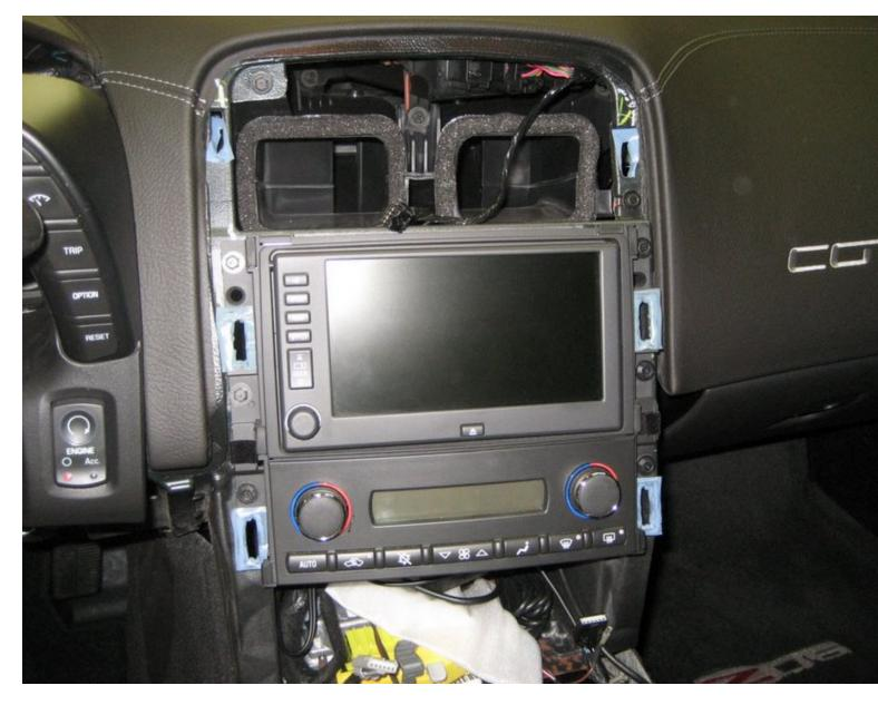
6. Once loose, you will need to disconnect the plugs for the seat heaters (if you have them), the cigar lighter and console power connector, the traction control switch, and the hazard warning switch.
