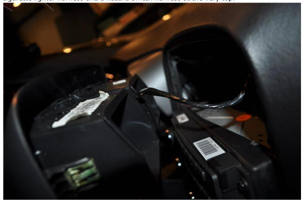
Once you've disconnected the connectors at the back of the bezel rotate it so the top of it goes toward the passenger seat and disconnect the remaining two wiring harnesses toward the back of the piece. The Active Handling/Traction Control connector is pretty much self explanatory. There is a plastic piece on the side of it that you gently pry up that will allow you to disconnect it.
