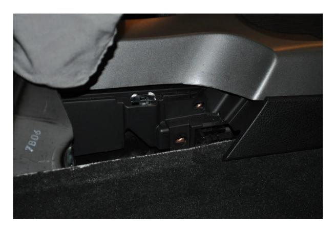
Carefully loosen the plastic trim piece that follows the radio bezel on the passenger side of the car. You don't need to take it all the way off, just loosen it as shown.
