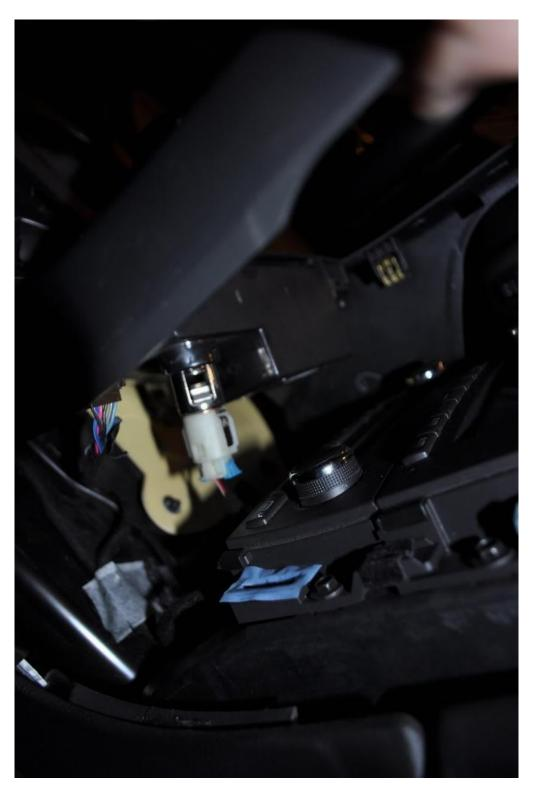
Once there are a few inches of clearance between the bezel and the dash, disconnect the wiring harnesses that connected to the back of it. Mine had two heated seat harnesses, a cigarette lighter harness and a hazard switch harness at the very top.
