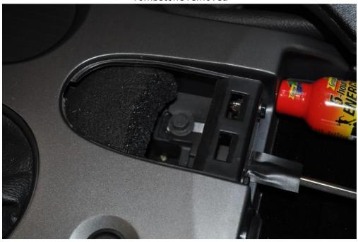
Remove the two 7 mm screws at the front of the center console.
