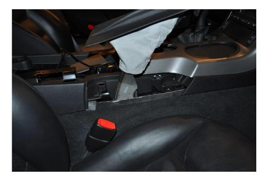
Remove the two 7mm screws that were exposed when the E-Brake boot was moved out of the way (shown below). Be careful not to drop the screws between the console and carpet.
