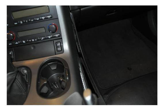
Lift the back of the center console off of the studs in the rear and slide it back towards the rear of the car. It may take some maneuvering to get it around the E-Brake boot.
