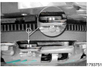
If the clearance between the rivet head (1) and the flywheel step is greater than 0.05 mm (0.002 inch), but is less than 6 mm (15/64 inch) at any of the three rivet head (1) and flywheel step locations, replace the flywheel only. Perform service procedure steps 2, 3 and 5.
