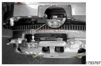
• The clearance between each of the three rivet heads (1) and flywheel step must be 6 mm (15/64 inch) or greater at all three locations. If the clearance between the rivet head (1) and the flywheel step is 6 mm (15/64 inch) or greater at all three locations, the flywheel does **not** require replacement. Reassemble the vehicle components and proceed to step 5. Refer to *Clutch Assembly* procedure for the 6.0L (LS2) engine or 7.0L (LS7) engine in SI.
