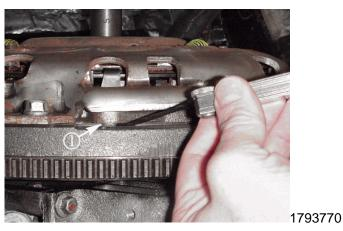
• If there is **less** than 0.05 mm (0.002 inch) clearance between any of the rivet heads (1) and flywheel step locations, the flywheel and clutch assembly must be replaced. Perform service procedure steps 2-5.
