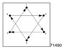
**IMPORTANT**: Remove the clutch pressure plate bolts in the sequence shown, starting with the number one and following in numerical order.
