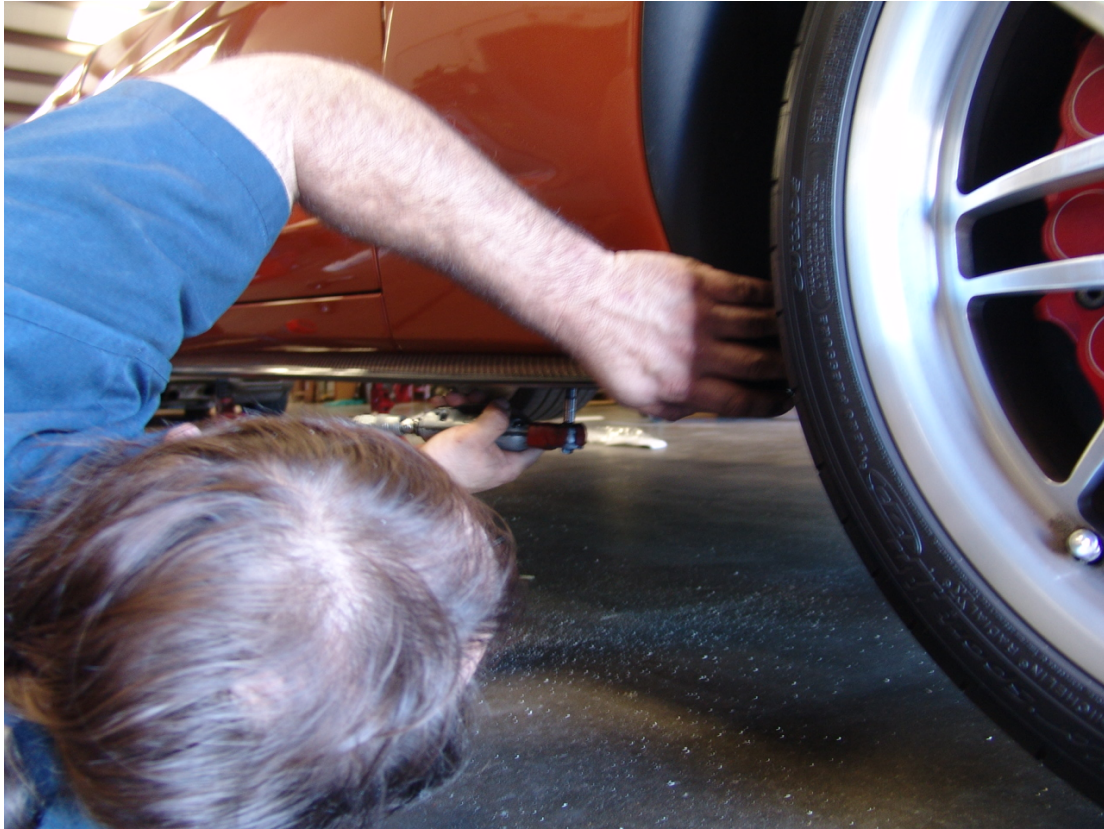
Figure 9: Final tighten of front lower bolts
