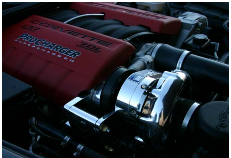
Completed ProCharger Installation
