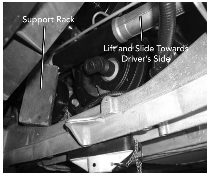
Rack Relocated for Balancer Bolt Removal
