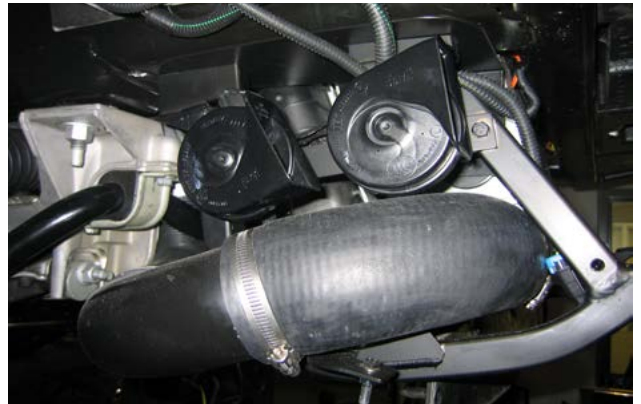
3" Rubber and Metal Elbow Installed
