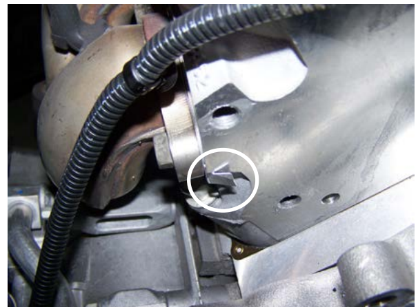
Exhaust Gasket Tab Removal
