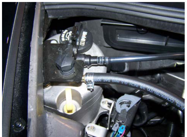
Hose attached to dry sump tank
