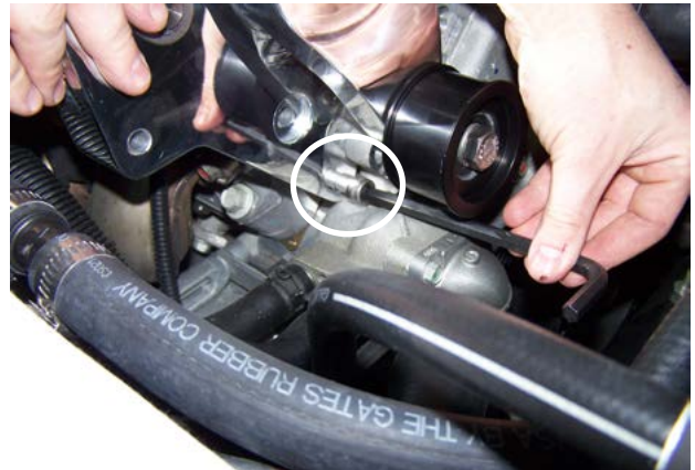
First Sub-Bracket Bolt Install
