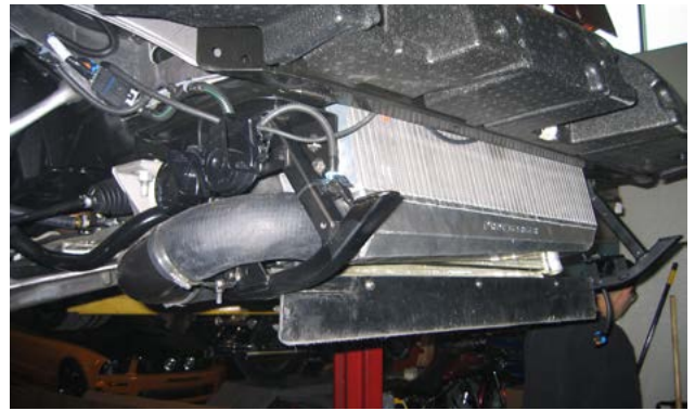
Intercooler and 3" Elbow Installed
