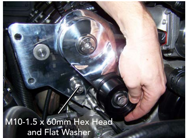
Sub-Bracket Mounting
