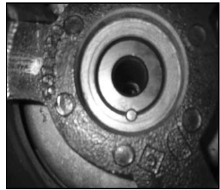
Harmonic Balancer Pinned to Crankshaft
